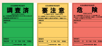
Stickers showing the results of the post-earthquake quick inspection of damaged buildings
